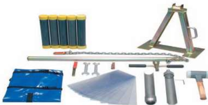
Fig: 1.4. SPLIT TUBE SAMPLER KIT Handle; short beating.; Split tube sampler; 2.08 in. ( 53 mm) ID x 15.74 in. (40 cm) length; Steel Hammer; w/nylon head caps 4.4 lbs. (2.0 kg) impact absorbing; Sample Liners; 1.97in. (50 mm) x 15.74 in. (40 cm) length; 10 pc; Plastic; Sample Liner retainers; Steel Lifting Jack; Lifting lever and wrap chain; Spanner .78 in. (20 mm) x 8.7 in. (22 mm) Bent Spatula; .78 in. (20 mm).
